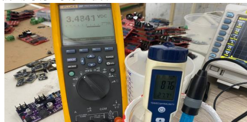
Figure 14. Test result of pH-Meter with digital multimeter
