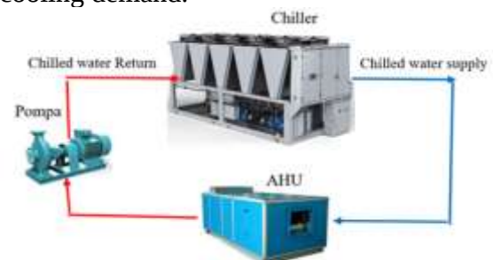
Figure 1. Chilled Water System
