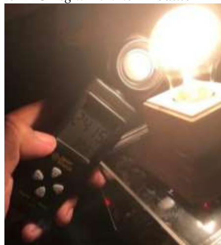
Fig. 13 Measurement using a lux meter
