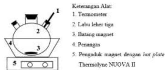
Gambar 1. Rangkaian alat adsorpsi sistem Batch
